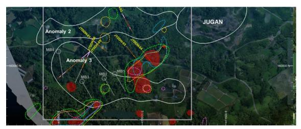
Figure 3: Drilling locations within the 2023-2024 Exploration DDH Program area relative to soil geochemistry anomalies; Au >0.018ppm (red polygon), As >54ppm (orange outline), Sb >16ppm (green outline), W >0.43ppm (blue outline) and Tl >0.18ppm (pink outline).
