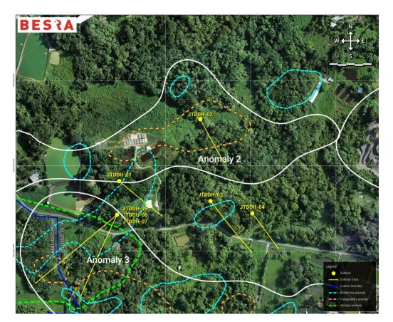
Figure 2: Drilling locations within the 2023-2024 Exploration DDH Program. The IP anomalies clipped to -50m depth. Chargeability (red polygons) and Resistivity (blue polygons). HyChips anomaly (yellow polygon) and 450hz DIGHEM resistor (dashed orange outline).
