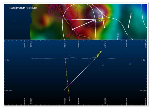
*Figure 5: Cross-sections along JTDDH-05, showing the zone of realgar and orpiment mineralisation and the 450hz DIGHEM Resistivity with the interpreted geological structure (dotted orange line).*
