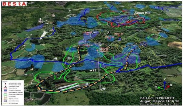
Figure 1: Distribution of IP geophysical anomalies (coloured pale blue) located to the west and northwest of the Jugan Hill, where the mineralised surface zone is highlighted in red. Green contours are boundaries of crystalline illite anomaly footprints.
