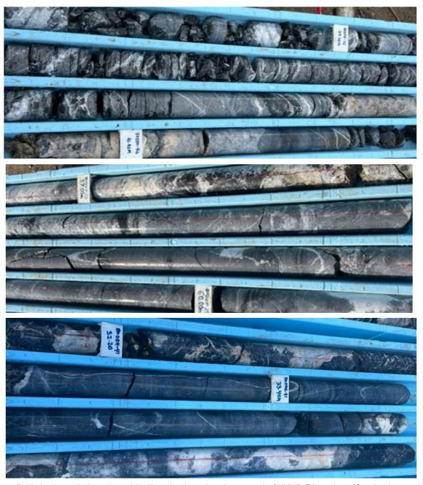
**Figure 5**: Hydrothermal alteration with silica dominated replacement in BKHHD-36 at circa 40m depth assaying gold grades of 5.60-10.7g/t Au (top); BKDDH-39 at circa 57m depth assaying gold grades of up to 13.03 g/t Au (middle); BKDDH-41 at circa 32m depth assaying grades of up to 14.21 g/t Au (bottom).
