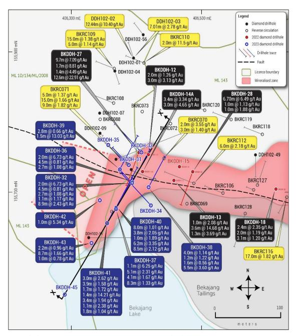
**Figure 1:** Significant drillhole intercepts from Besra's DDH 2022-2023 programs (black – first round, blue – follow-up round) superimposed onto historical Resource wireframe (in puce) along portion of the northern flank of the Bekajang tailings dam. Section XX' is shown in Figures 3 & 4.
