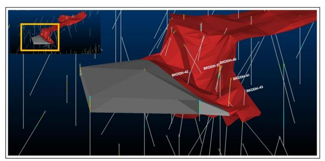
**Figure 6:** 3D model showing mineralisation (in red) and potential for possible extension (in grey) together with historical drill holes having significant Au intercepts.
