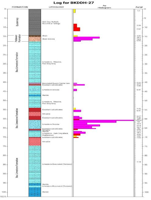
**Figure 2**: Summary of core lithology and gold assay results for BKDDH-27 showing exceptional gold tenor within two distinct intervals; at the LSC and deeper within the Bau Limestone.
