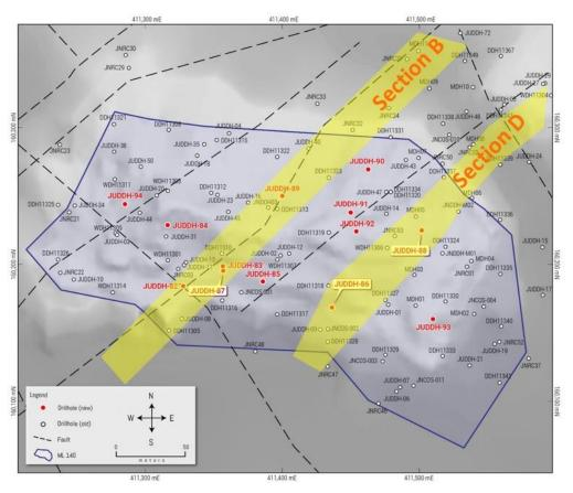
**Figure 4:** Showing the location of the 2021-2022 Jugan diamond drilling program, highlighting the locations of JUDDH-86 to -88 and the approximate locations for Sections B & D shown in figures 5-6 & 8-9.
