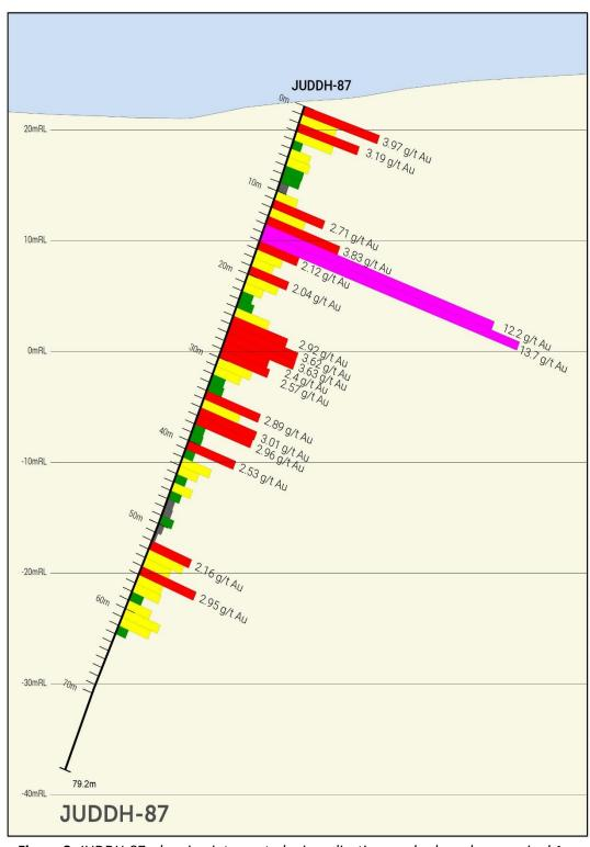
**Figure 2**: JUDDH-87, showing intercepted mineralisation grades based on nominal 1m sample widths. Note that the intercepted thicknesses are not true thicknesses because of the inclined trajectory of the drill core – See Appendix 1.
