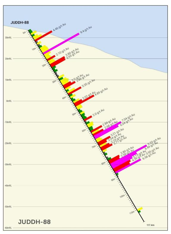
**Figure 3**: JUDDH-88, showing intercepted mineralisation grade and thicknesses based on nominal 1m sample widths. Note that the intercepted thicknesses are not true thicknesses because of the inclined trajectory of the drill core – See Appendix 1.
