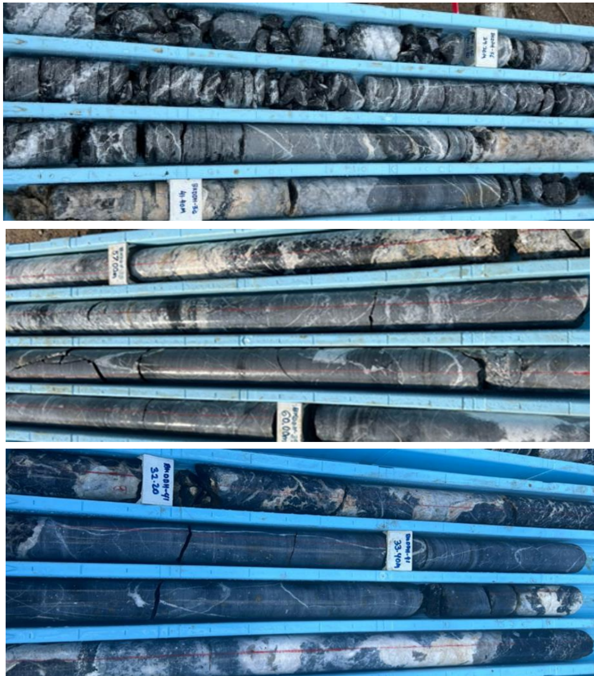
Figure 5: Hydrothermal alteration with silica dominated replacement in BKDDH-36 at circa 40m depth assaying gold grades of 5.60-10.7g/t Au (top); BKDDH-39 at circa 57m depth assaying gold grades of up to 13.03 g/t Au (middle); BKDDH-41 at circa 32m depth assaying grades of up to 14.21 g/t Au (bottom).
